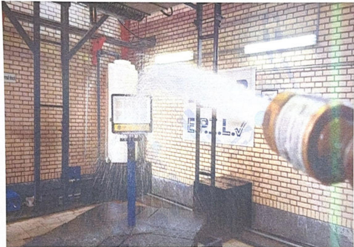
Figure 3: EUT under IPX6
