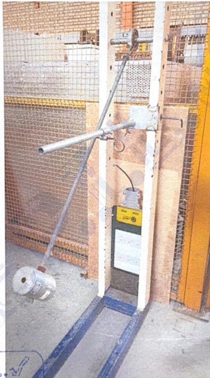
Figure 5: EUT under IK10
