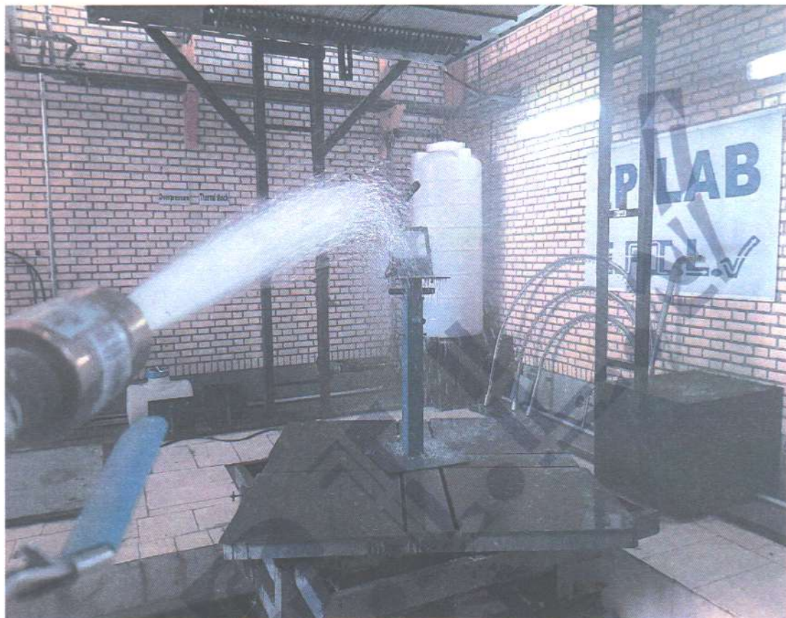
Figure 3: EUT under IPX6
