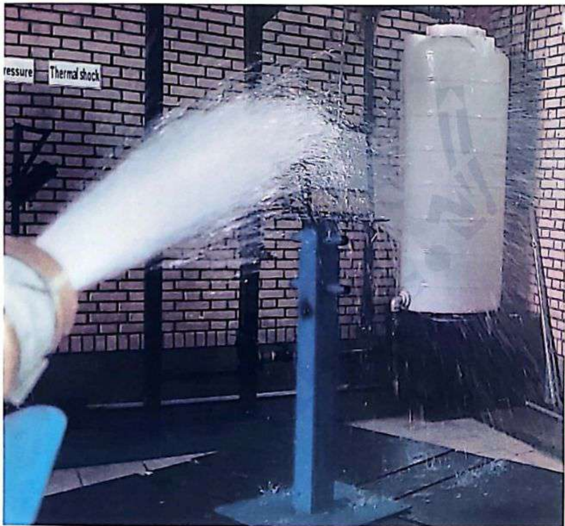
Figure 3: EUT under IPX6
