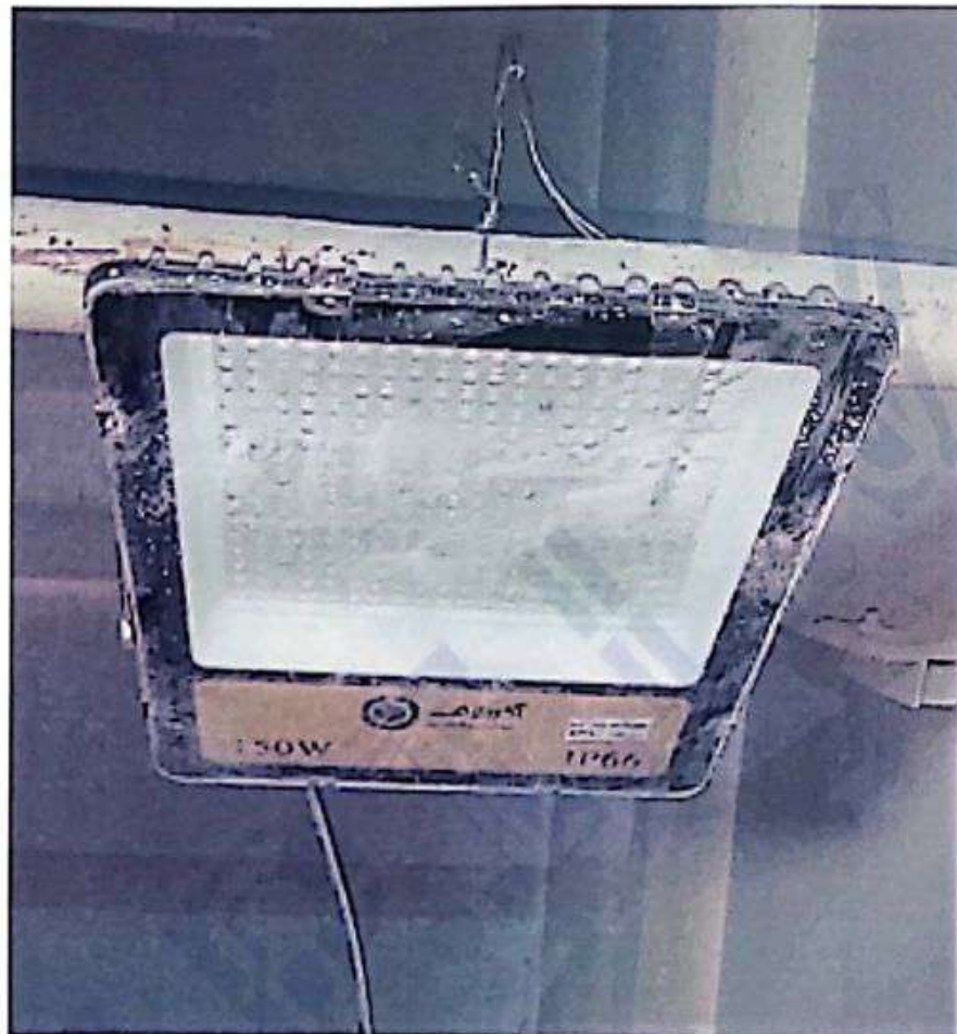
Figure 2: EUT after IP6X
