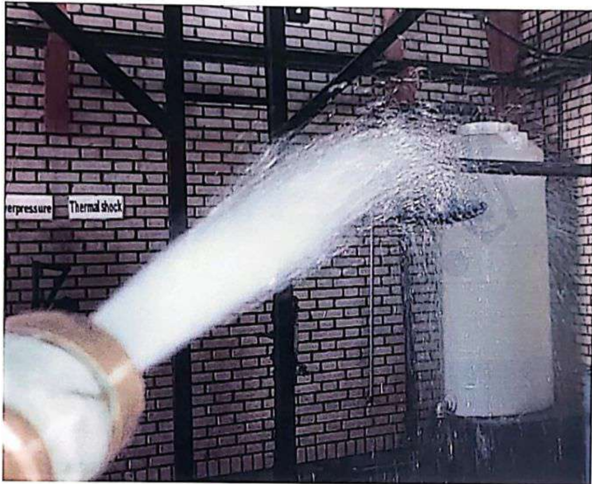
Figure 3: EUT under IPX6
