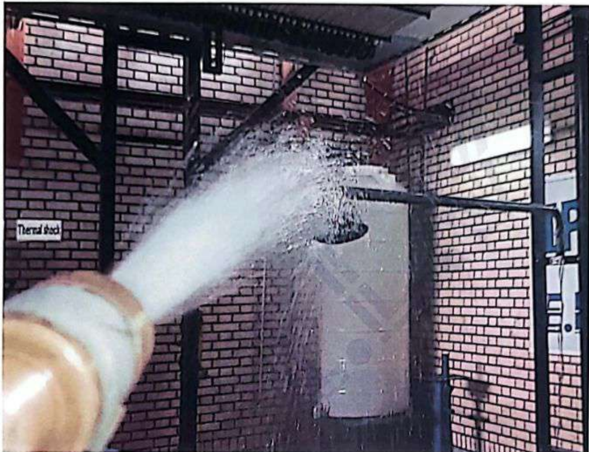
Figure 3: EUT under IPX6
