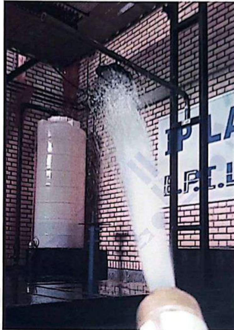
Figure 3: EUT under IPX6
