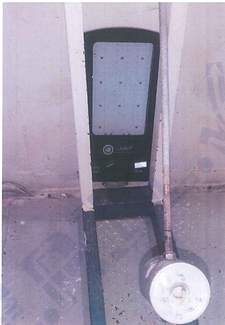
Figure 2: EUT under IK08
